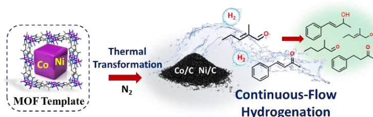
Figure 1. Schematic illustration of catalyst synthesis and the hydrogenation process.
